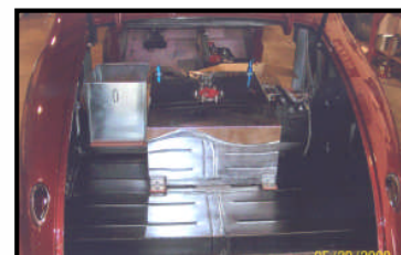
Custom aluminum fuel cell, battery box and a tool box are shown looking in from the rear of the car.
